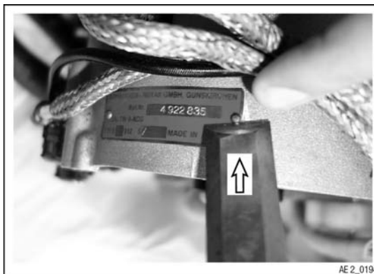
Fig. 3 Remove of the grooved pin
